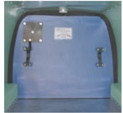
SAFETY NET: An insulated bulkhead used to protect temperature in a van body has a little more intricate design than the typical bulkhead .
